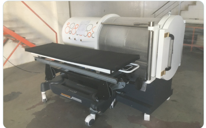
Steel monoplace chamber with acrylic tube section and patient transfer stretcher.
